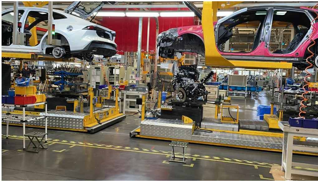
Figure 13 – The “marriage”, an assembly part of a chassis and body.
